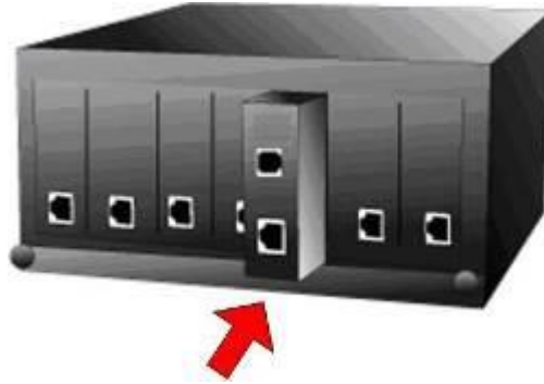
Figure 3-3: Insert a VDSL2 Bridge into an available slot
